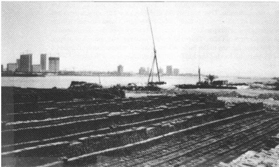
Figure 2 - Present day brick manufacturing in Egypt. Sun drying of bricks before going through the kiln. Little has changed in this process from ancient to present day Egypt.
